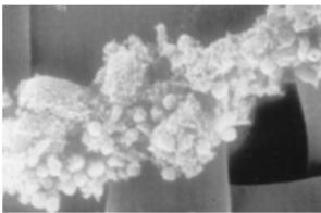
Electron Micrograph of microaggregate on a 40µm screen
